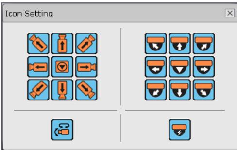
With click in icon setup window, you can set direction of camera. Icons for sensor and alarm can not be set.
