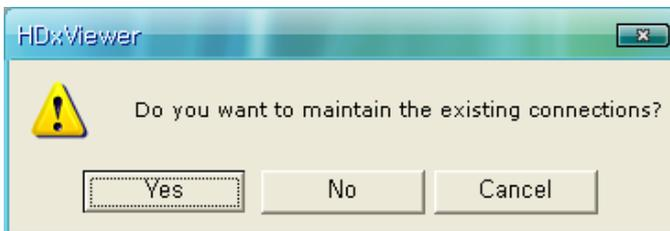
If user wants to keep maintaining the existing connection, HDxViewer display layout changes to 64 channel view. In addition, newly added DVR cameras will be display right after the existing cameras.
