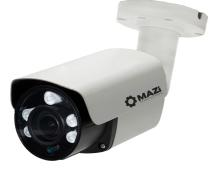
IP Bullet Camera 2MP, 1080P/2.8 12MM 2MP Φ14 AF/5pcs array IR/audio I/O, hardware reset, POE High performance CMOS image sensor, with 2 MP resolution H.264/H.265, dual-stream Max Resolution 1920\*1080 Onvif ICR switching IP66 metal bullet casing 5 pcs Array IR LED, 40 m 2.8 ~ 12 mm/AF lens Power supply: PoE and DC12V 550 mA 1 CH AUDIO I/O, Support hardware reset
